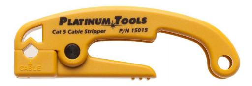
Designed for stripping the cable jacket on Category 5, 5E cables twisted pair cables • Will not nick inner conductors • Durable high impact plastic housing is molded from yellow plastic to make it easier to locate • No adjustments required • Long life blade
