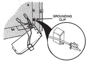
Feed electrical power cable through open knockout in corner of housing and attach with appropriate connector. Allow 6" of wire inside of housing.
