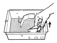
1. Slide the wiring cover out of housing.
