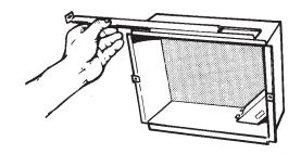
Choose which side of housing will be mounted directly to a wall stud. Then, insert the mounting bracket, from the opposite side, and into the channel at the top of housing.
