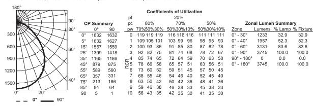
**2GTL 4 40L LP835**, 4006.7 delivered lumens, test no. LTL22798PO, tested in accordance to IESNA LM-79.
