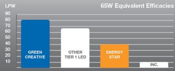
At 81 LPW, this lamp's efficacy is more than 20% higher than the Tier 1 LED BR30 65W replacement industry average and exceeds ENERGY STAR requirements by upwards of 100%. This energy-saving performance makes this lamp a smart retrofit choice for incandescent bulbs.
