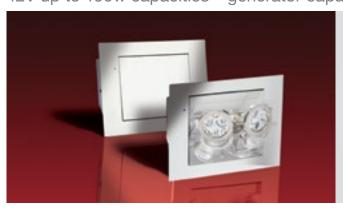
Designed for architectural applications, the Phantom<sup>™</sup> Series stays hidden until needed. In normal conditions (stand-by) the emergency light is concealed in the wall or ceiling. In case of power failure, the door of the unit rotates open 180° and exposes the emergency light. When main power returns or at the end of the discharge period, the light turns off and the door rotates closed automatically.
