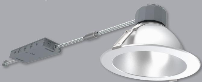
**Mechanical** - SPECFIT retrofits existing commercial housings. Spring action clips to accommodate ½" to 2" ceiling thicknesses. Fixture with remote driver installs and is accessible from below the ceiling.
