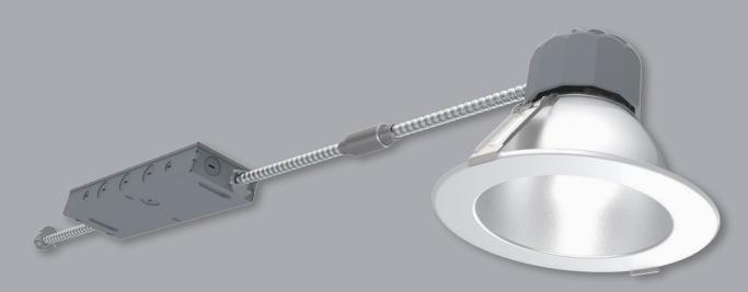
**Mechanical** - SPECFIT retrofits existing commercial housings. Spring action clips to accommodate ½" to 2" ceiling thicknesses. Fixture with remote driver installs and is accessible from below the ceiling.
