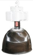
16" or 22" High Bay Prismatic: Indoor fixtures for use above 25'. 16" unit for 250w Pulse Start Metal Halide, 22" unit for 400w Pulse Start Metal Halide. Die cast aluminum housing and wiring box. Clear acrylic Lexalite Reflexor prismatic refractor. Ballast and lamp supplied.
