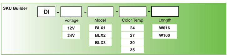
Example: DI-12V-BLX2-27-W016 = Diode LED, 12 Volt, Wet Location BLAZE™ X, Type 2, 2,700° CCT, 16.4 foot spool.
