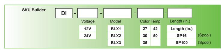
Example: DI-12V-BLX3-27-SP16 = Diode LED, 12 Volt, BLAZE™ X, Type 3, 2,700° CCT, 16.4' spool.
