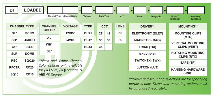
Example: DI-LOADED-SQBL-24V-BLX3-CL-36-CV = Diode LED, Fully Loaded, Square, Black Channel, 24 Volt, BLAZE<sup>TM</sup> X 300, Clear Lens, 36 inches, 96" Lead Wire, and with a Constant Voltage Driver.
