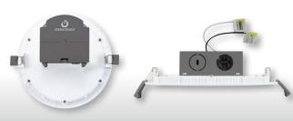
The 6" GOOF RING is designed specifically for use with THINFIT Series 6" NEW CONSTRUCTION DOWNLIGHT 11.6W fixtures. The 6" GOOF RING increases the trim diameter to 8.67" and is ideal for covering mistakes or when the ceiling hole is larger than the fixture.
