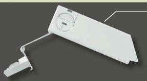
Open Wide keeps the fixture open and your hands free to wire. By simply pressing the wiring compartment holding tab, the wiring compartment cover swings down and out and stays in position until you're ready to snap it back in its closed position and slide the lens back in place.
