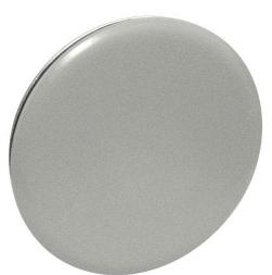
3-1/2" steel, screw/bar type knockout seals are inserted in discontinued, open box knockouts to protect exposed wires. They are used in oil tight applications when they have gaskets. Garvin Industries' one piece preassembled screw and backer bar slides on open knockout holes without removing box devices or covers.
