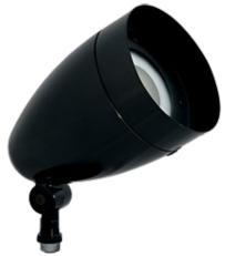
Bullet shape die cast aluminum flood with 13 Watt LED Light Engine. Comes with flood reflector installed. Optional spot reflector included for field installation.
