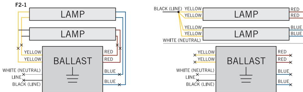
2. Confirm that the lampholders in the fixture are R17d Double Recessed Contact lampholders. These DirectDrive LED tubes require R17d Double Recessed Contact lampholders.
