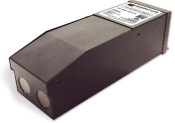
Magnitude's M100L12DC-AR is the most compact LED driver on the market with a magnetic transformer core. It is equipped with two auto-reset breakers, one on the input and one on the output, which protect both the load and driver. The driver is encased in a coated metal. box that includes 2 knock-outs, to enable easy installation that complies with electrical code requirements.
