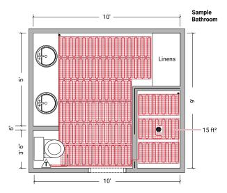
Select the Mesh kit that is no larger than the heated area. The heated area is the area of the floor that does not include permanent fixtures such as cabinets, toilets, sinks or tubs. The selected kit can be configured on the jobsite to fit the shape of the area to be heated.
