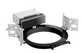
Easy to install 4" and 6" rough-in with die-cast aperture ring, removable driver, thermal protector and adjustable butterfly brackets. This rough-in is designed to make new construction recessed downlighting easy 90 CRI.
