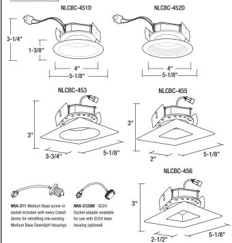
Source: 12W Chip on Board 1000Lm LED (845 Delivered)
