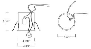
Cut out: 4-5/16" Height: 4-1/4" Housing Length: 4-3/4" Housing Width: 4-3/4"
