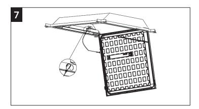
8. Close the retrofit kit door into the fixture and rotate the clips to secure the door closed.
