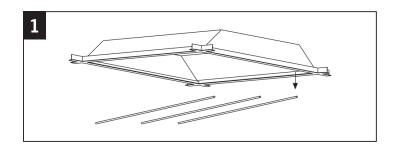
2. Insert the two brackets into the clearance between the housing and T-grid.
