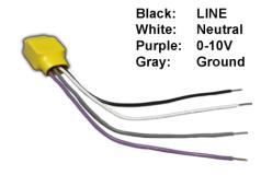
Warning: Version 1.0 of the Receiving Module must be connected with LINE and NEUTRAL correctly. In Version 1.0 the Neutral and the DIM(-) are internally connected. Failure to connect correctly could cause line voltage to be present on the dimming circuit.
