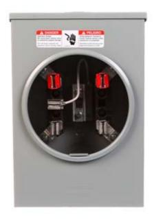
Siemens Low Voltage Talon Meter Sockets Residential - Talon Meter Sockets UAT1 Steel are Residential Enclosures Single-Family Metering. Type: UAT1 Special Features: NO BYPASS Application: RESIDENTIAL Standard: UL Voltage Rating: 300V Amperage Rating: 135A Phase: 1 OR 3 PHASE Size: 5.000X8.800X13.400 Cable Entry: OH Terminal: 5 TERMINALS Mounting: SURFACE MOUNTING Operating Temperature: AVERAGE AMBIENT Enclosure: STEEL
