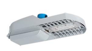
LED roadway lighting that replaces up to 250W MH or 150W HPS. Optics are factory installed and meet IES Distribution Type II.
