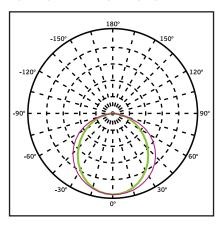
$\label{eq:maximum Candela} \begin{aligned} &\text{Maximum Candela} = 1525.2 \\ &\text{Located at Horizontal Angle} = 0, \\ &\text{Vertical Angle} \ 0 \end{aligned}$
