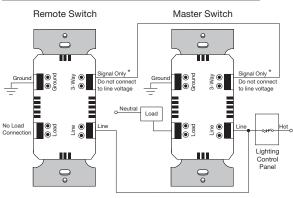
Each switch wired for multiway operation has the ability to turn on, turn off or override a shutoff signal.
