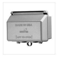
Receptacle Covers - Weatherproof - WeatherBox Metal While-In-Use Covers Meets 2005 NEC Article 406.8 (B)(1) for receptacles in damp or wet locations. Diecast powder coated aluminum. NEMA 3R rating. Comes with gasket, mounting hardware, duplex receptacle insert and GFCI receptacle insert. Lockable to prevent accidental disconnects.
