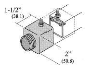
Conduit entry fitting with 1" NPT male thread on 9/16" long nipple. Fits 1-5/8" (41.3) square channel only. Comes complete with FF-100 stud nut assembly.
