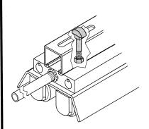
3/8"-16 X 2-1/4" shoulder bolt with special head to fit through P3S channel slots. Bolt extends 3/4" (19.1) below 1-5/8" (41.3) square channels. Hex nut included.
