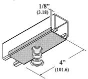
Spacer fits between channel and electric discharge lighting fixtures where 1/8" (3.2) clearance is required. Clearance hole for EB-22 wiring nipple nut also shown on this page. (Nipple and locknut not included.)
