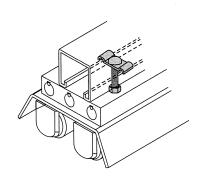
1/4"-20 x 1-1/4" stud nut for fixture attachment. Stud extends 1" (25.4) below channel slot. Hex nut included.
