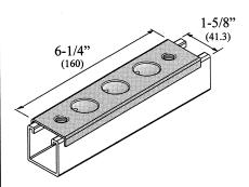
Outlet plate fitting. Three 7/8" (22.2) dia.K.O.'s on 1-3/16' (30.2) centers. Supplied ready to install with VN-1025 channel nuts and 1/4" x 5/8" flat head machine screws.
