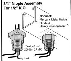
This adaptor works with manufacturers standard 1/2" K.O. raceway channel or VF-7105-A fixture hanger. 3/4" male pipe thread nipple can be removed if 3/4" female
