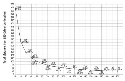
Number of LED MiniDisc per lead NOTE: No more than 200 LED MiniDisc Lights per LEDDR-12-60W.
