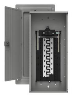
SIEMENS LOW VOLTAGE ES SERIES LOAD CENTER. FACTORY INSTALLED MAIN BREAKER WITH 30 1-INCH SPACES ALLOWING MAX 30 CIRCUITS. 1-PHASE 3-WIRE SYSTEM RATED 120/240V (100A) 22KA INTERRUPT. SPECIAL FEATURES: ALUMINUM BUS, GRAY TRIM, NEMA TYPE1 ENCLOSURE FOR INDOOR USE. REPLACED BY SN3030B1100. AVAILABLE 4/1/2020
